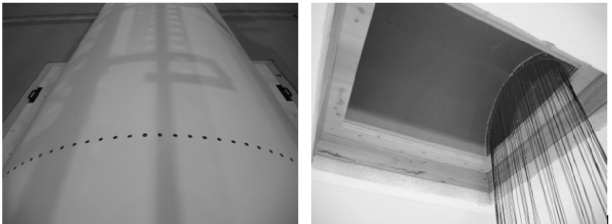
Figure 6.9: Flush-mounted microphones on the rigid open half cylinder. Left: view in chamber 1 in Fig. 6.5. Right: view in chamber 2 in Fig. 6.5.
