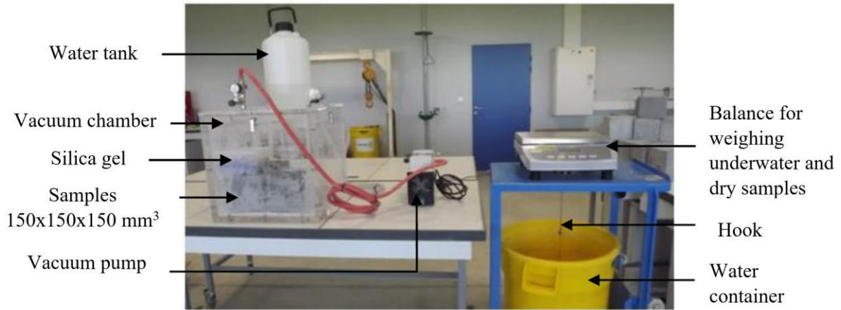
Fig. 4. Device for measuring porosity and apparent density [120].
