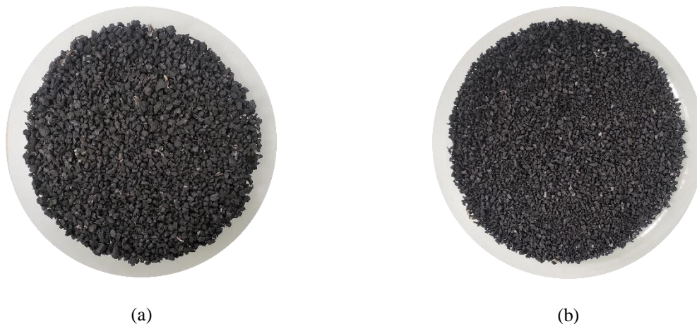
Fig. 2. Two sizes of recycled tire aggregate: (a) coarse (1.6-10 mm), (b) medium (1-4 mm).
