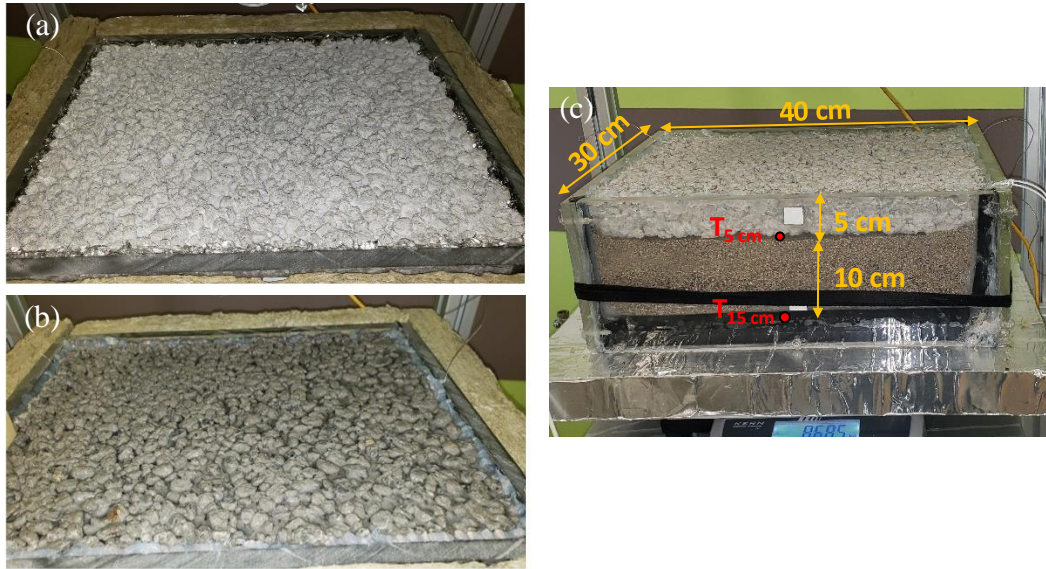
Fig. 5. The placement of PCP1 in the bin: (a) dry condition, (b) wet condition, (c) the dimensions of the complete PC pavement structure.
