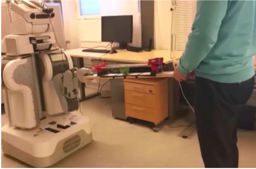
Figure 3.2: A human-robot collaborative team. Each agent holds an edge of a gutter on which there is a ball [9]. They try, for instance, to position the ball in the center of the gutter.
