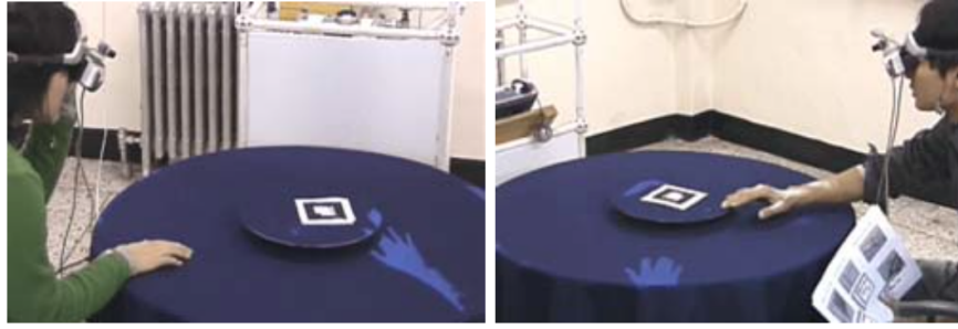
Figure 2.7: Virtual shadows of a collaborator's arms are displayed on the surface of a table. Figure from Sakong and Nam [197].
