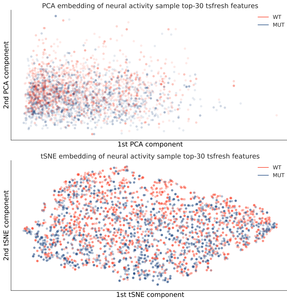
Figure 5-1 – Top: Scatter plot of a two-dimensional PCA embedding of the motor cortex activity time-series encoded by top-30 tsfresh features (with features sorted by importance scores determined from a random forest classifier trained on the dataset). The class labels are color-coded with red points corresponding samples from control animals and blue points to samples from mutant ones. Bottom: similar scatter plot of the top-30 tsfresh features of neural activity time-series embedded with a t-SNE algorithm.
