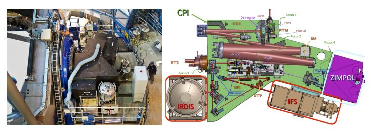
Figure 1 – The SPHERE instrument (Beuzit et al., 2019), pictured in the top-left image, is composed of an ExAO system, powerful coronagraphy and three instruments: the IFS, the ZIMPOL and the IRDIS instruments (seen in the top-right figure) (source: de Boer, J. et al., 2020).
