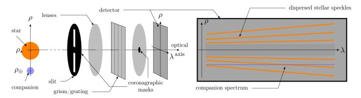
Figure 3.1 – Schematic of an LSS instrument (left) and the data it's collecting on the detector (right), in high-contrast imaging. Wavelength ( $\lambda$ ) and angular separation to the coronagraphic mask's center ( $\rho$ ) are indicated.
