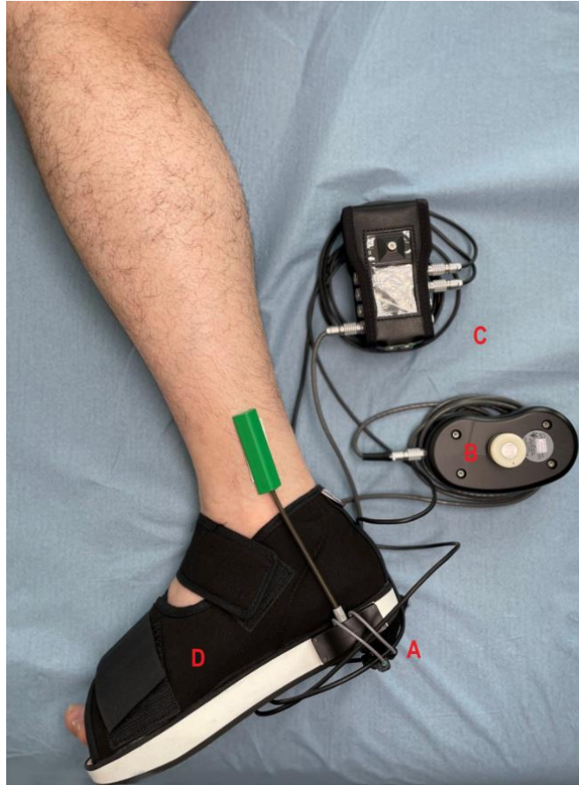
Fig 1. Equinometer with its various components: A= Electronic twin-axis goniometer, B= MyoMeter electronic dynamometer, C= DataLOG D= Rigid shoe.
