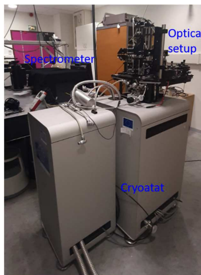
Figure 2.14 Photo of the Magneto-optical spectroscopy setup. The optical setup is installed just above the cryostat. The excitation source and the detection pathway are connected to the setup with an optical fiber. A superconducting magnet up to 9 T is integrated inside this cryostat.
