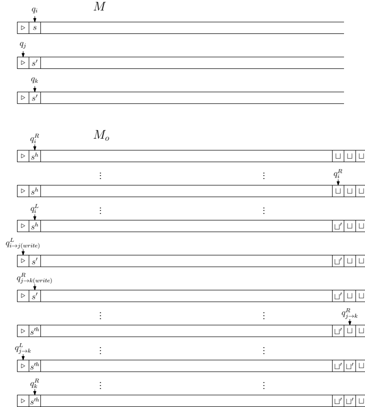
Figure 2.6: Description of the M_o simulation when the head of M is at the first cell.
