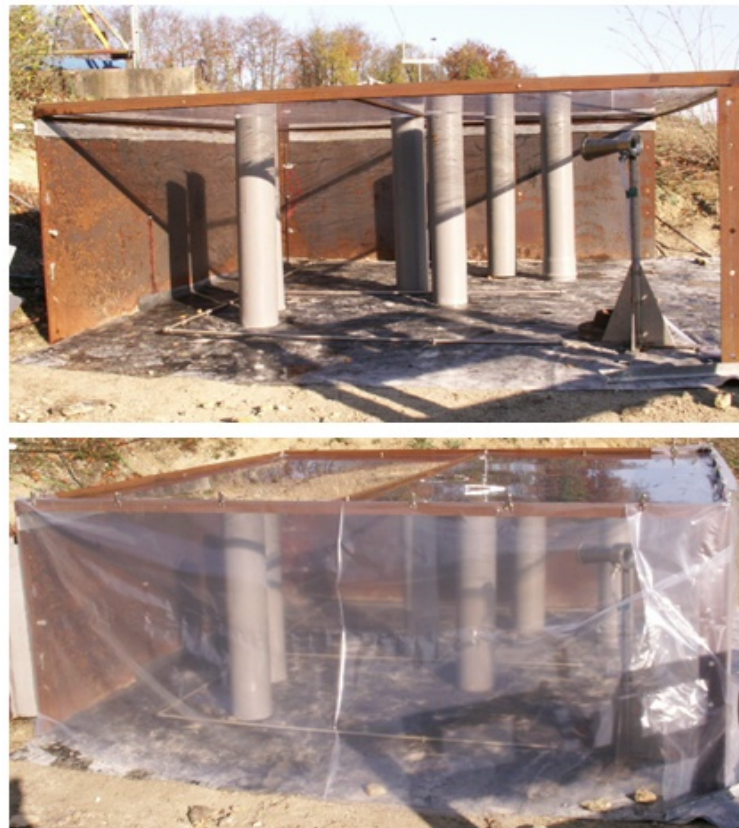
Figure 3-87: Schematic representation (and photograph) of experimental setup used to investigate the propagation of a hydrogen- air flame in an obstructed media
