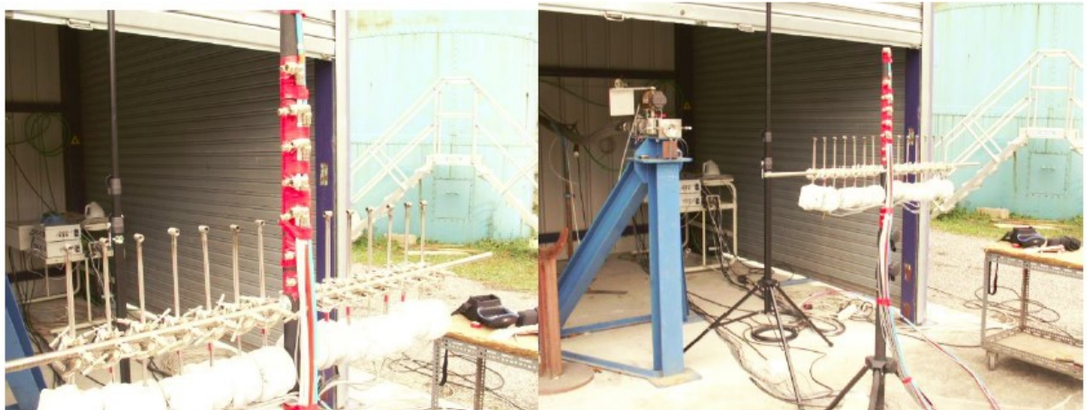
Figure 3-29: Measurement masts (velocity and concentration sensors, the orifice manifold is located on the blue pillars)
