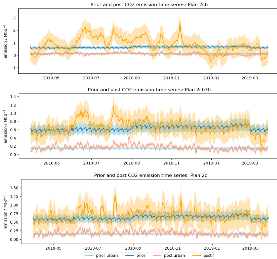
Figure 4.24 The daily emission fluxes before and after inversion of Plan 2cb (whole-block) , Plan 2cb30 (30-day block) and the reference Plan 2c, compared to observations, with shade of InterQuartile Range.
