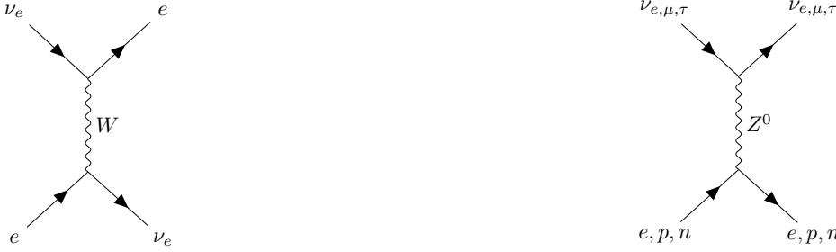
Figure 1.10: Tree-level Feynman diagrams of neutrino interactions due to charged current interaction (left) and neutral current interaction (right).
