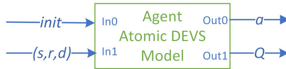
Fig. 7.1 The DEVS agent atomic model with its two input ports In_0 and In_1 used to receive the initialization message (for the Q matrix) and the set (s, r, d) from the DEVS environment model. The two output ports Out_0 (resp. Out_1 ) are used to send the action a (resp. Q matrix) to be evaluated by the environment model.
