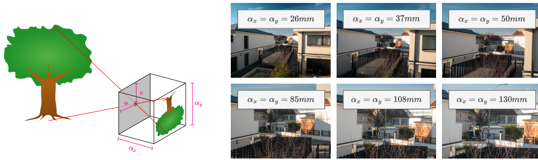
(a) The intrinsic parameters. \{\alpha_x, \alpha_y\} is the focal length. \{u, v\} is the principal point. Figure modified from [88]. (b) Impact of different focal lengths \alpha on the image.
