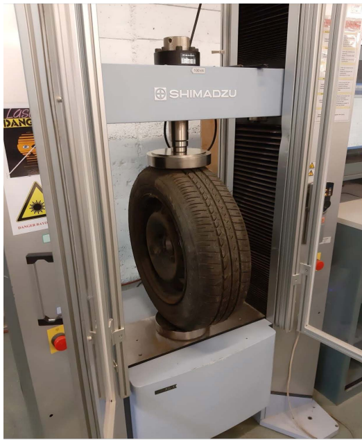
(a) Tire compression test
