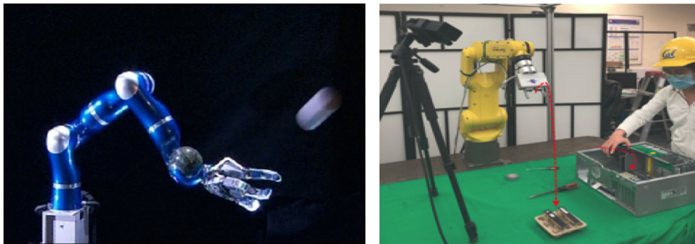
(a) The robotic arm catching a ball thrown to it [136]. (b) Robot and human collaborate to assemble a desktop [137].
