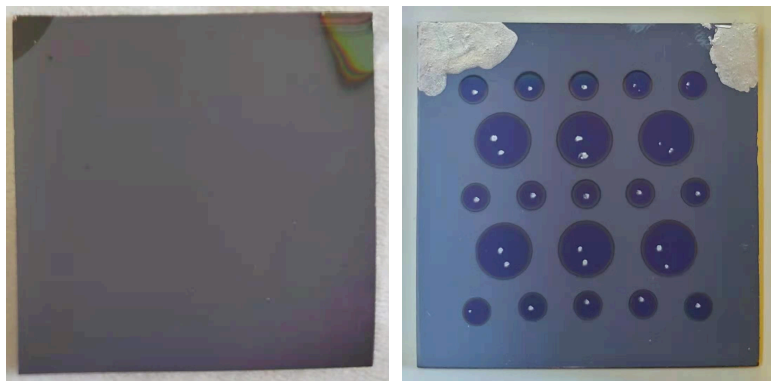
Figure 2.10 Photographs of solar cell before and after ITO deposition through shadow mask (16 cells with ITO pad area of 0.0314 cm 2 , 6 cells with ITO pad area of 0.125 cm 2 ).
