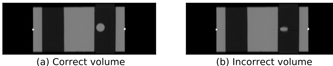
Figure 2.1: Example of incorrect volume reconstruction because of motion during a conventional CT scan. The phantom is static but the tumor in the left lung is moving during the acquisition. The correct volume of the tumor is shown in (a), and the reconstructed volume is shown in (b).
