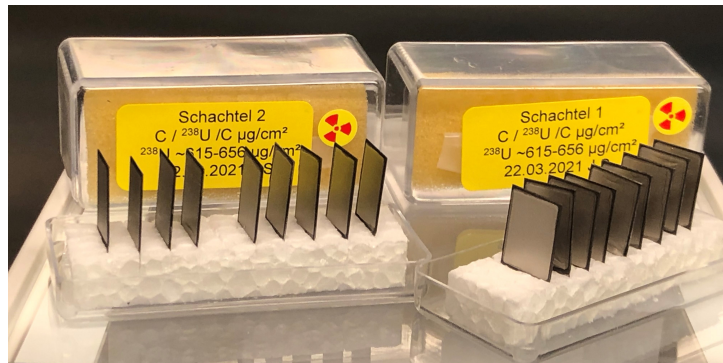
Figure 3.4: The metallic ^{238}\text{U} targets sitting in two plastic boxes with dimensions of 70 \times 35 \times 30 \text{mm}^3 for transportation. Photograph taken by Bettina Lommel, GSI.
