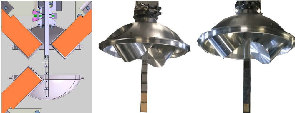
Figure 3.3: Left: Schematic illustration of the target holder, and the top and bottom hemispheres of the target chamber with 3 LEPS detectors, described in Section 3.4.2, inserted through the doigt de gant (see text for details). The part of the target chamber to which the beam line and the VAMOS++ spectrometer connect is not shown. Middle and right: Photographs of the top hemisphere and the targets mounted on the target holder in and opposite of the beam direction, respectively. Numbering of the targets is from bottom to top. The Al degrader is placed behind the targets #2, #3 and #4.
