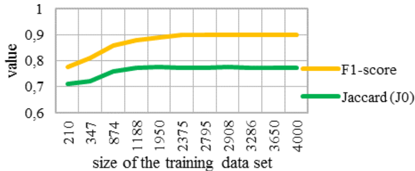
Fig. 51. Variation in the network performances according to the size of the training data set.
