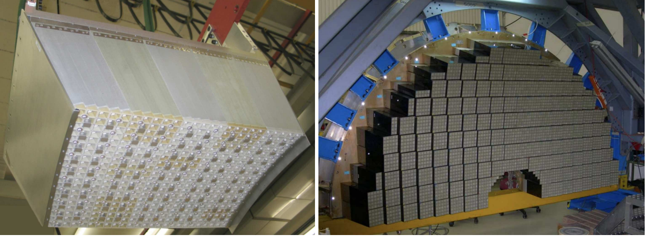
Figure 2.7: Left: Front view of an ECAL module equipped with crystals. Right: An endcap Dee of the CMS ECAL, fully equipped with supercrystals. The figures are taken from [43].
