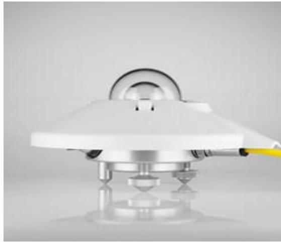
Figure 13: CM6B pyrometer (WMO 2008)
