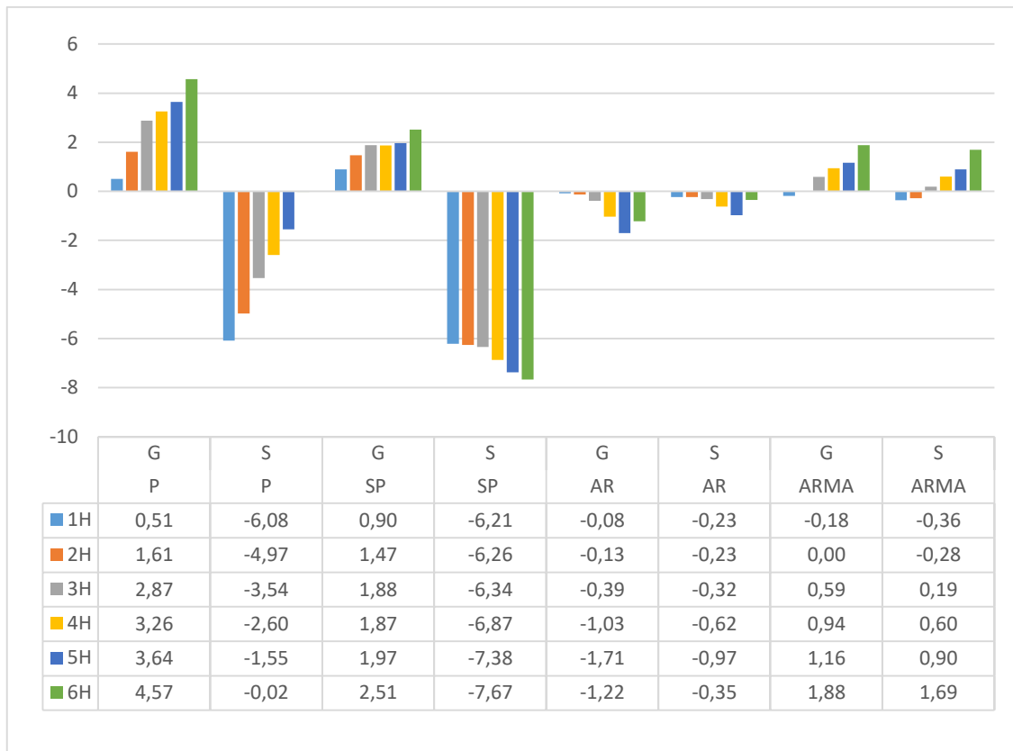
Figure 36: nMBE forecasting errors vs. Horizon for Ground measurement (G), Satellite-derived data (S) with four statistical models in 2016.
