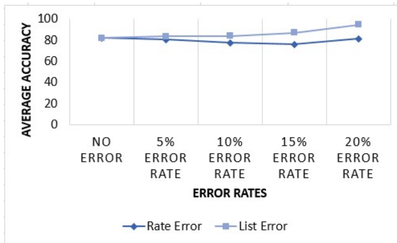
Figure 5.7: Accuracy in Leakage Detection from all nodes
