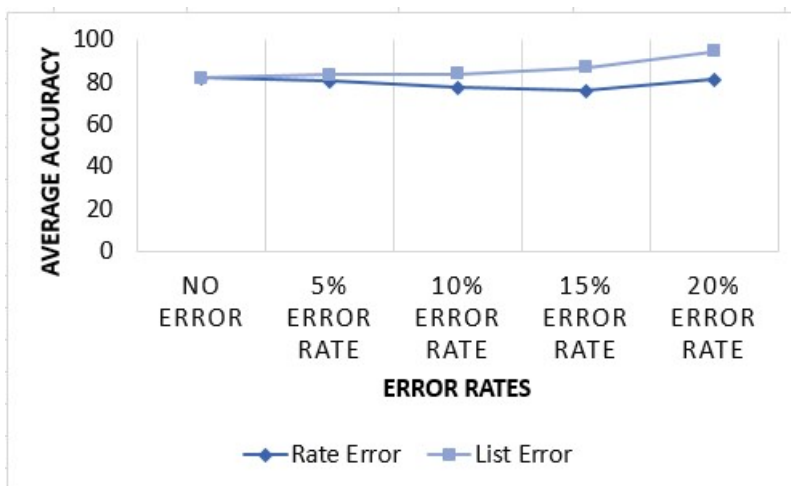
Figure 5.7: Accuracy in Leakage Detection from all nodes
