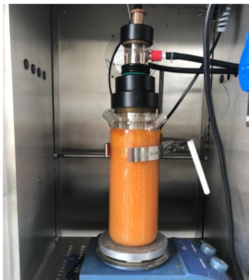
Figure 35. System used for preparation of the final compounds, at end of reaction with precipitated product stirred in iodine-colored ethyl acetate.
