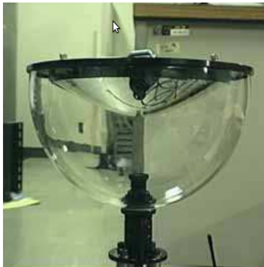
Figure 2.33: A hyper omni vision omnidirectional camera. The camera combines a perspective camera and a hyperbolic mirror. The prototype was developed at Osaka University, Japan. This image is courtesy of Yagi et al.
