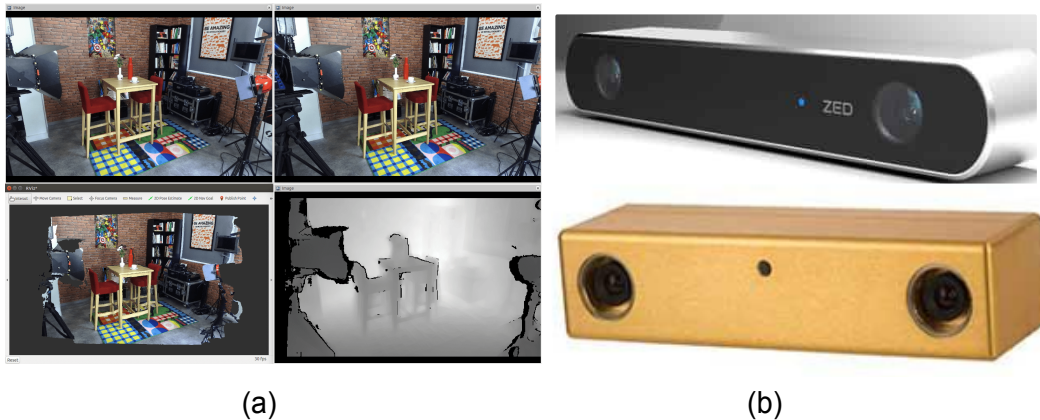
Figure 2.23: The ZED (top) and Bumblebee (below) stereo vision cameras. The new generation stereo vision camera captures high-resolution images. On the left are images captured from the ZED camera that display high-resolution from both left and right cameras, the 3D point clouds, and disparity image.
