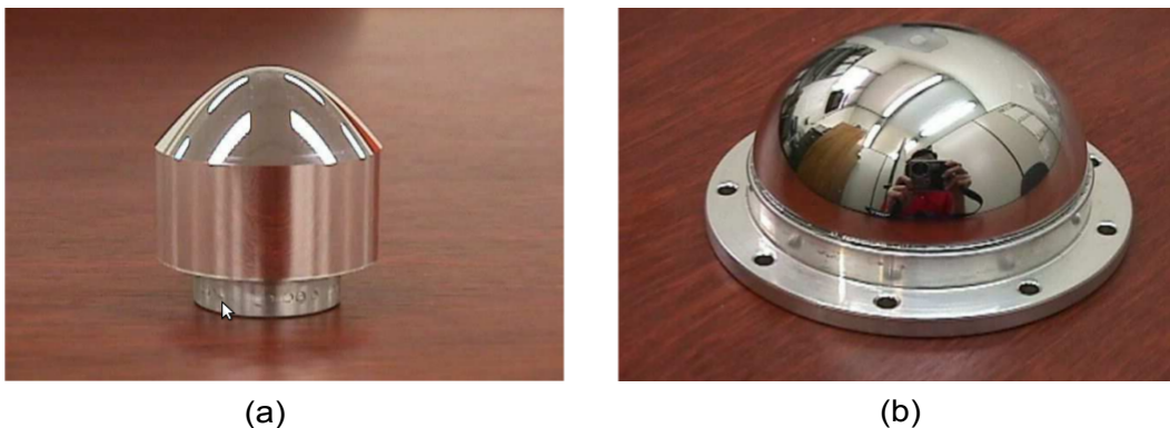
Figure 2.32: Conic mirror. Hyperbolic mirror (a) and spherical mirror (b) manufactured using aluminium metal. They are formed using high precision CNC lathe machine. High spindle rotation and low feed speed can produce a smooth and shiny surface. The image is courtesy of Grassi et al.
