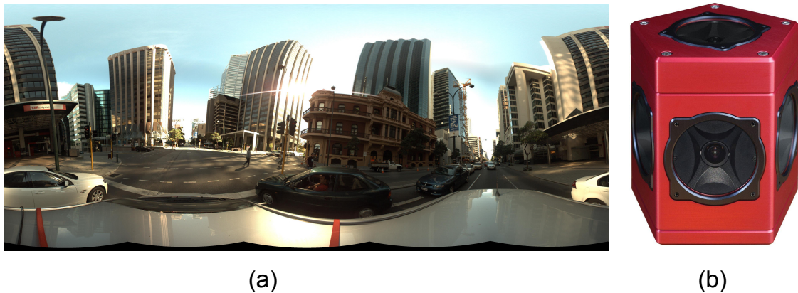
Figure 2.18: The polydioptric camera consists of six cameras. Five cameras are used to capture horizontal images and produce 360° horizontally, with one capturing the upper image. (a) shows the panorama image stitched from five images. (b) The image is the commercial polydioptric camera, LadyBugs from Point Grey.
