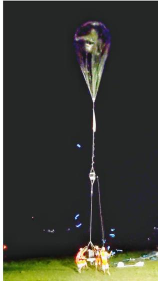
Figure 1.10: Picture of a balloon launch during the first scientific campaign of Strateole-2. The gondola is carried by the technical teams until the balloon can carry it entirely to avoid impacts with the ground.
