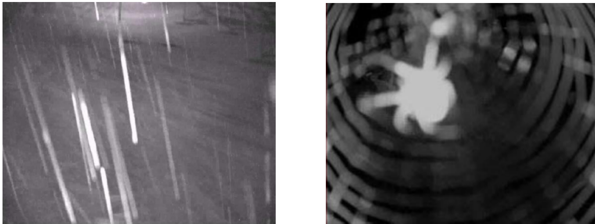
Figure 1.1: Issues with the infrared camera: low visibility in rain (left) and insect on camera (right).
