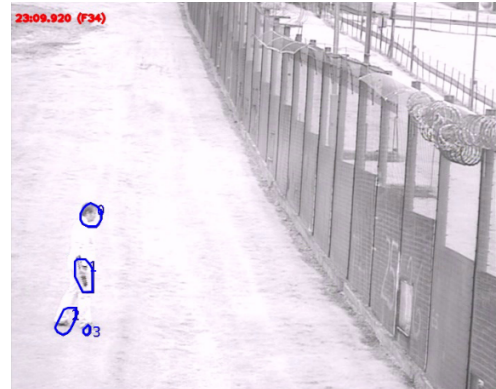
(b) Object split into extra detections in i-LIDS dataset. Blue blobs show split-object detections along with their index number.
