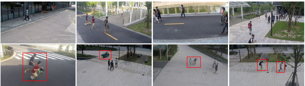
Figure 1.7: Some frames from the ShanghaiTech dataset, each from different scene. First row contains frames without any anomaly but with different scene dynamics. Second row depicts the following anomalies in red bounding boxes (left to right order): chasing, small truck, brawling and two people jumping.
