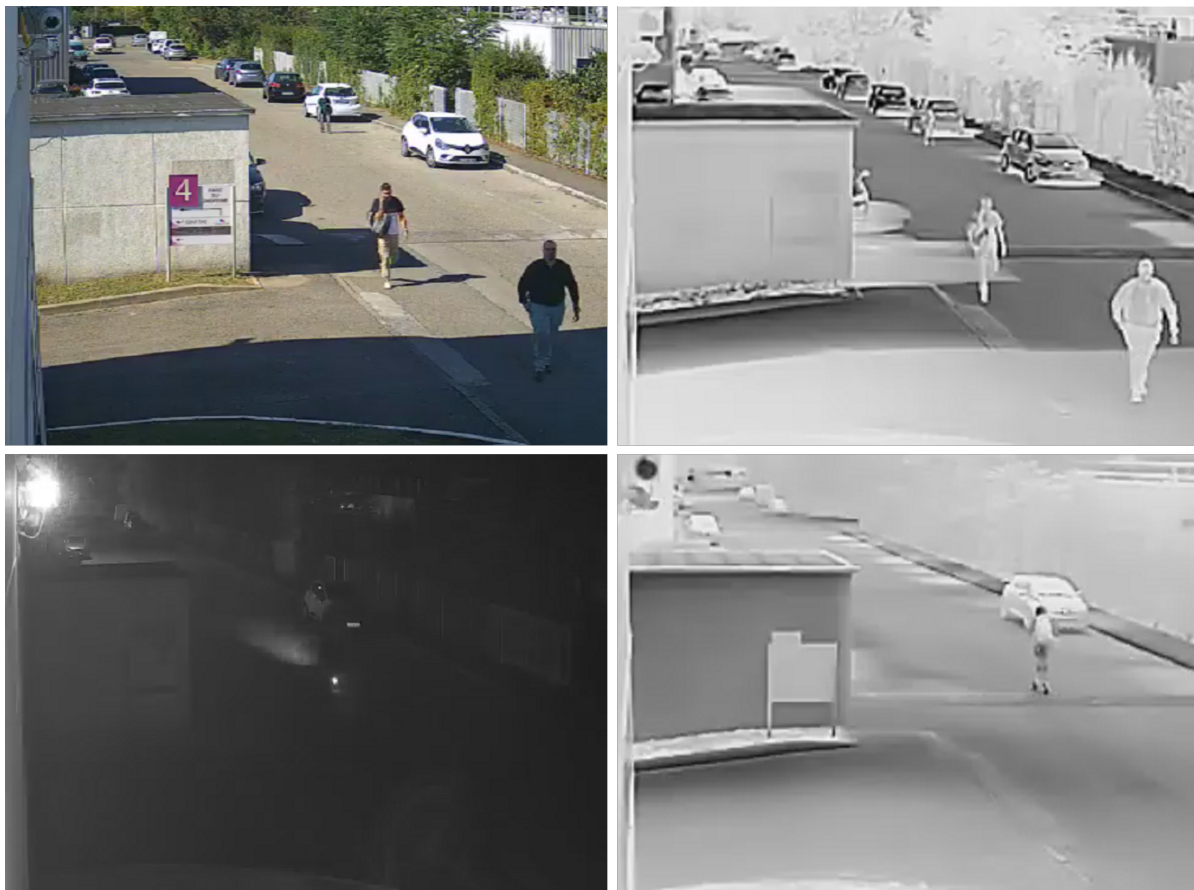
Figure 1.2: Data acquisition on a site by color (left) and thermal camera (right). Each camera captures two scenes at the same instant, one during day (top row) and the other during night (bottom row).
