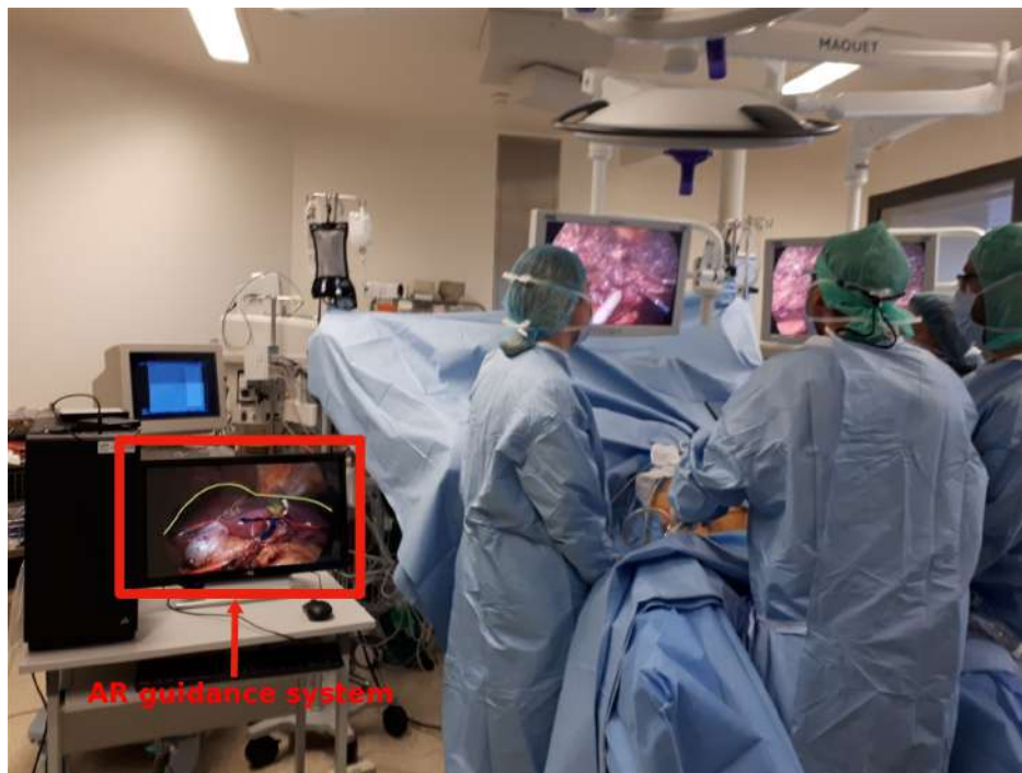
Figure 4.3: Usage of our AR guidance system (left computer) in the operating room to perform a laparoscopic tumour resection.
