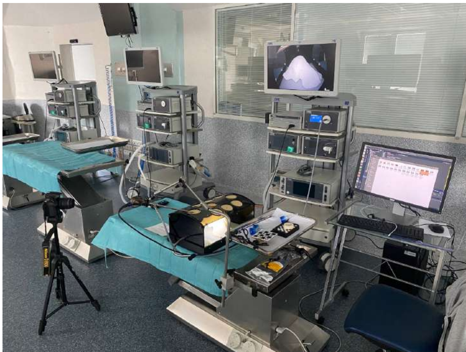
Figure 6.8: Setup for keyhole estimation experiments using phantom data. At the left of the image: The external camera used to measure the pointing errors. Center: The pelvitrainer with the liver phantom and the laparoscope fixed with a mechanical arm. Right: the PC with the AR software connected to the endoscopy system.
