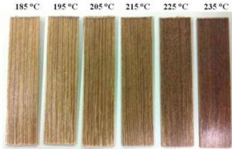
Figure 1-25. The effect of molding temperature on jute/PLA composite with temperature range of 185, 195, 205, 215, 225, 235 °C and at a constant 20 bar pressure [110]
