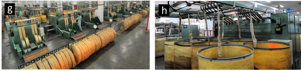
Figure 2-3. Drawing-in of jute fibers, machine back (g) and front (h)
