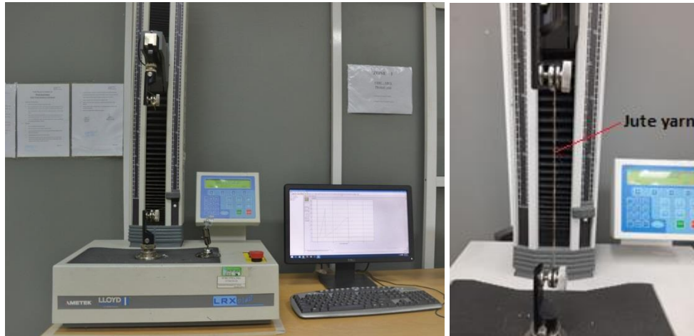
Figure 2-26. Single yarn testing machine (Lloyd Ametek)
