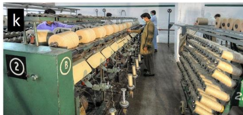
Figure 2-3. (k) Winding of jute yarn [138]
