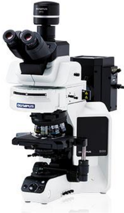
Figure 5-4. Olympus BX 53 refractive microscope, resolutions range 40-1000 x
