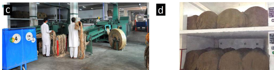
Figure 2-3. (c, d) Lubricating and pilling of jute batches
