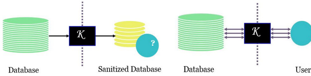
(a) Interactive: Multiple Queries, adaptively chosen (b) Non-Interactive: Data are sanitized and released Figure 8: The two approaches to release the DP and BP outputs: interactive and non-interactive.
