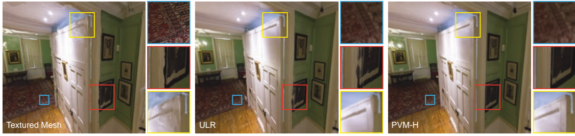
Figure 3.4: Textured mesh preserves sharp details in diffuse regions that are lost due to blending in ULR and PVM-H (blue inset). ULR corrects minor geometric errors in textured mesh typically in glossy regions (yellow inset). Large geometric errors, such as ones due to occlusion edges, are rectified by per-view geometry improving PVM-H rendering quality over ULR (red inset).
