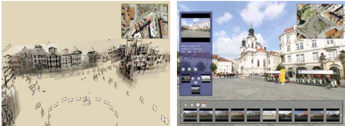
Figure 2.5: The first interactive Image Based Rendering (IBR) system, PhotoTourism, was proposed by Snavely et al. [2006] which allowed a user to interact and navigate smoothly between photos of a landscape collected by crowdsourcing.
