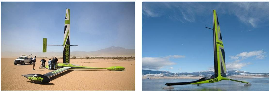
Figure 234. The Greenbird, a wind-powered car, breaks the speed record in the Nevada desert at 201 km/H, piloted by the Englishman Richard Jenkins. It also uses a rigid carbon sail of the Foil type to reach 3 to 5 times the wind speed.
