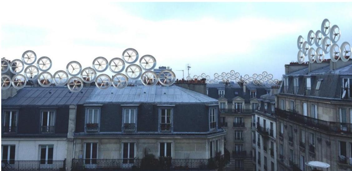
Figure 253. Visualization of flag clusters on a Parisian building (Horizontal and vertical). This device captures the winds induced by the corridor effect of dense and homogeneous fabric streets , but is too "foreign" to the architecture present.
