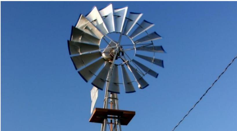
Figure 289 Pumping wind turbine
