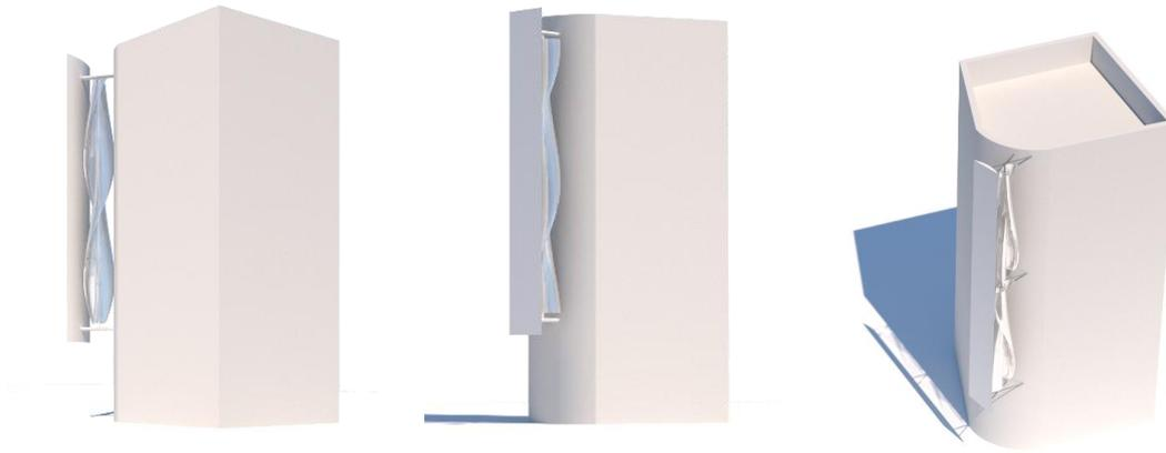
Figure 170 3D studies of a 45° aerofoil on a rounded corner of a building
