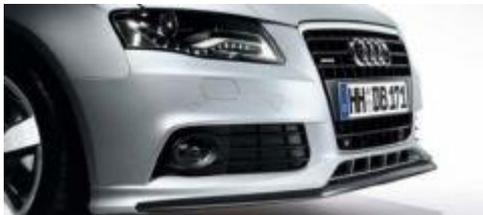
Figure 240 Examples of DTM blades on the front of a car
