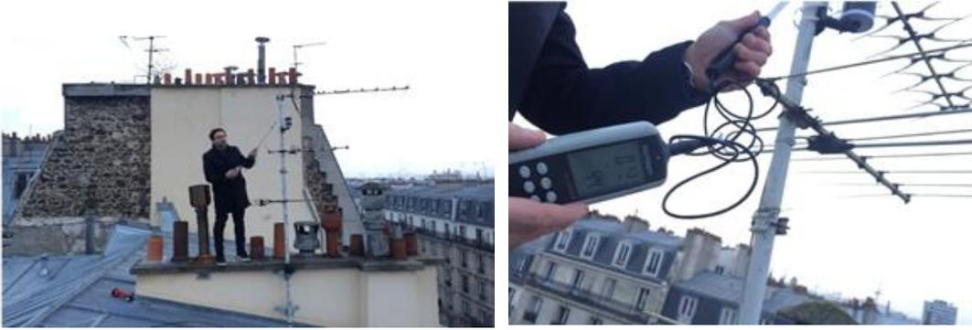
Figure 192 Figure 191: Installation of the anemometer on the roof of the building 136 avenue Parmentier, Paris 11ème. A TV antenna was used to support the device.
