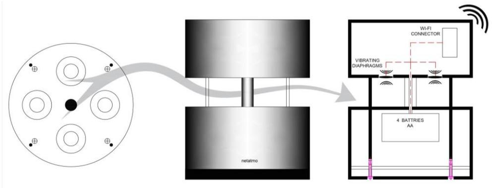
Figure 85. Plan, elevation, cross section of the anemometer used
