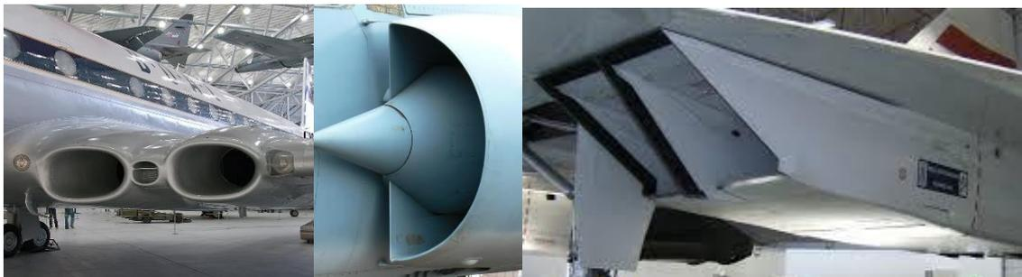
Figure 227 Examples of air intakes on the fuselage of a jet aircraft
