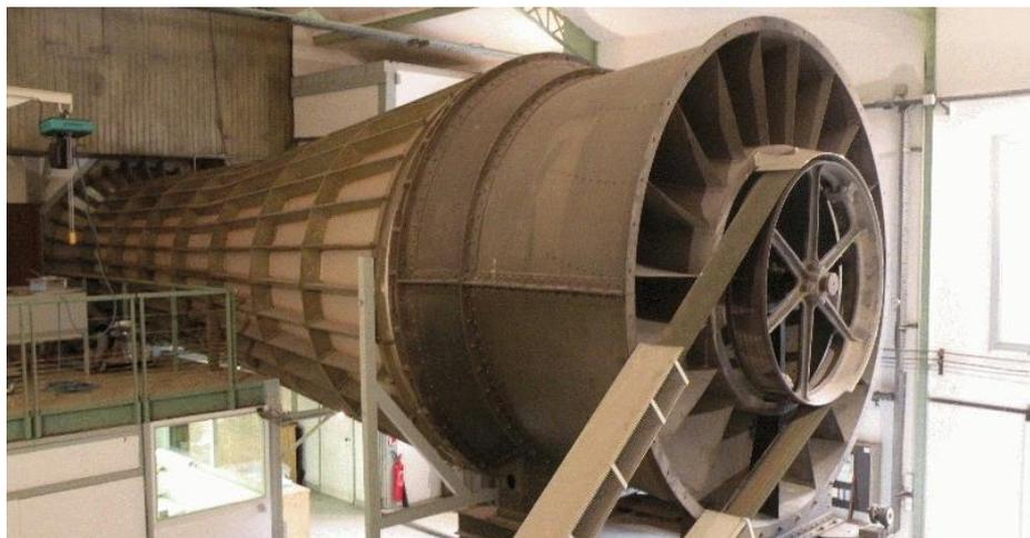
Figure 25. Motorization of the Eiffel wind tunnel, Photo D. Serero of 18/09/2016 . Source © Laboratoire Eiffel, courtesy of Mr. Martin Peter
