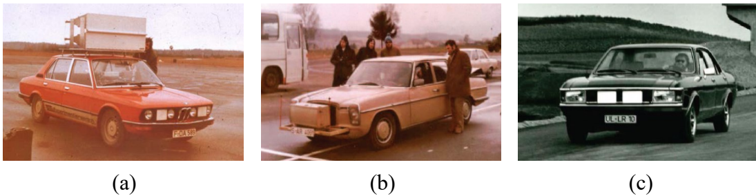
Figure I.1.11 Early automotive radar systems. (a) 10 GHz radar in the early 1970s. (b) 16 GHz radar in 1975. (c) 35 GHz radar in 1974.
