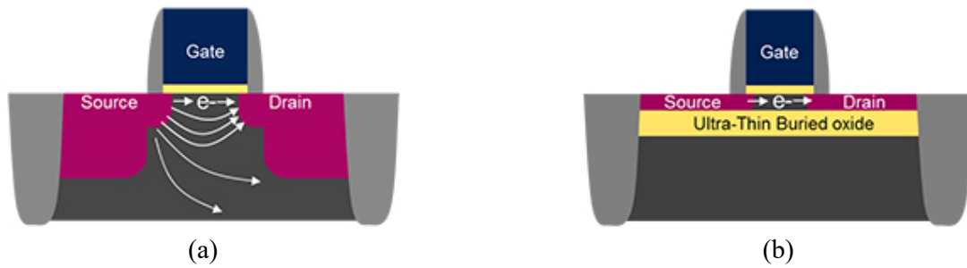
Figure II.1.2 (a) Bulk CMOS versus (b) FD-SOI. (Source: STMicroelectronics).
