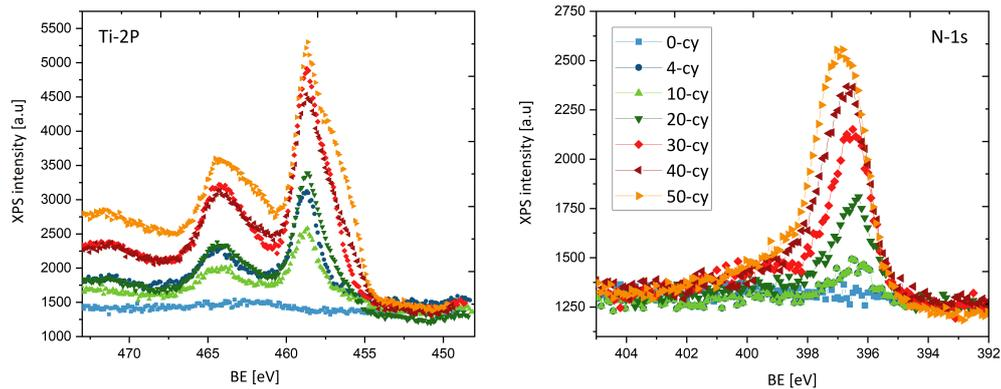
Figure 6.9: The XPS Ti-2p and N-1s core level spectra of the TiN-Al<sub>2</sub>O<sub>3</sub> coated Si samples with the number of TiN ALD cycles from 0 to 50
