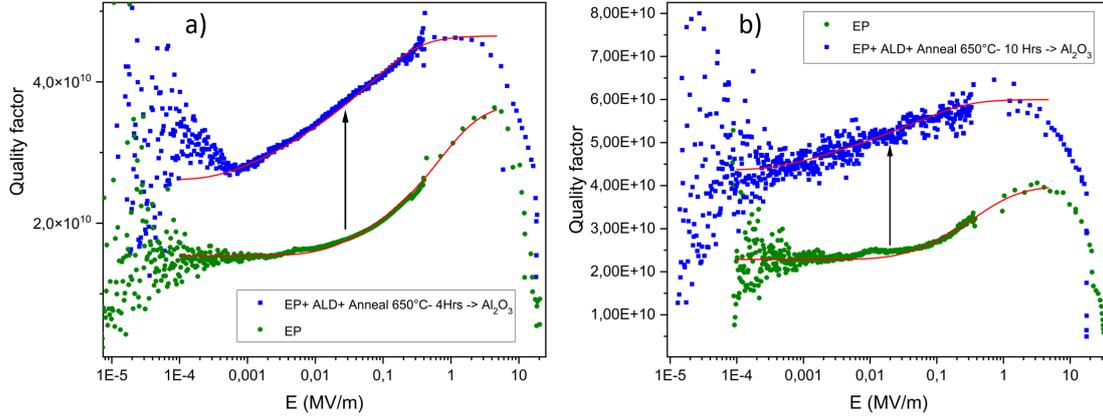
Figure 5.22: Tests  $Q$  vs  $E$  at 1.5K in the low field regime on a Nb cavity coated with  $\text{Al}_2\text{O}_3$  (10 nm) and post annealed at  $650^\circ\text{C}$  for (a) 4 hours and (b) 10 hours.
