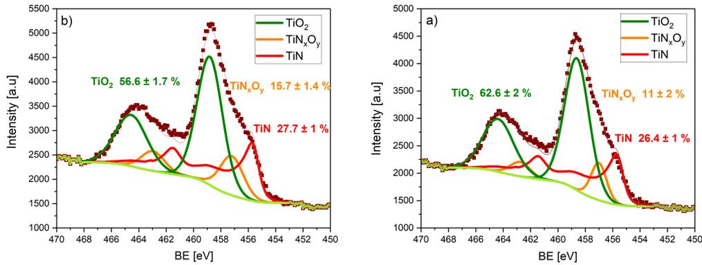
Figure 6.15: Composition of the 40 cycles TiN film: (a) as deposited (b) after conditioning with 400 mC/mm<sup>2</sup> dose
