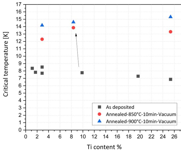
Figure 7.16: The critical temperature of the NbTiN films after different annealing treatments measured on sapphire substrates
