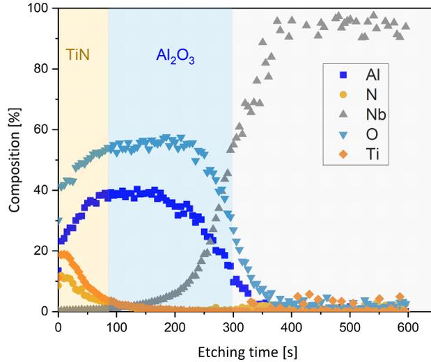
Figure 6.19: XPS depth profile of TiN-Al<sub>2</sub>O<sub>3</sub>-Nb sample after annealing at 650°C during 10 hours under vacuum
