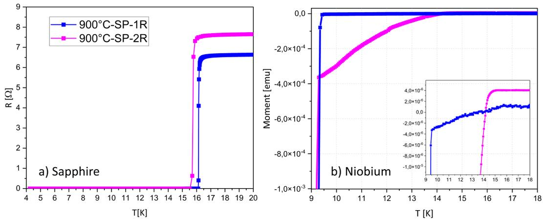
Figure 7.30: Critical temperature measurements on the NbTiN film (6:1)
