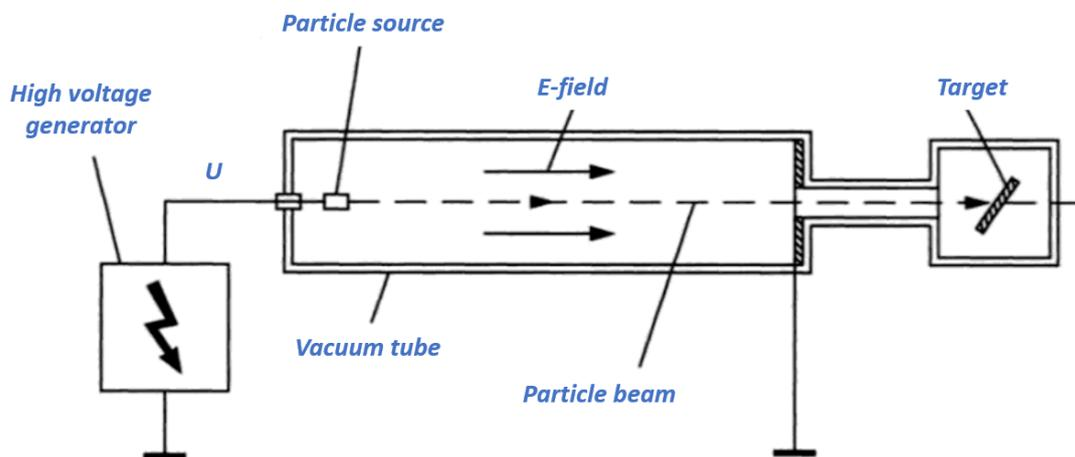
Figure 1.1: Illustration of the direct-voltage accelerator (figure after [2])
