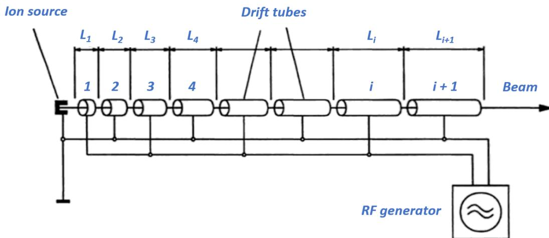
Figure 1.2: Illustration of Wideroe accelerator (figure after [2])
