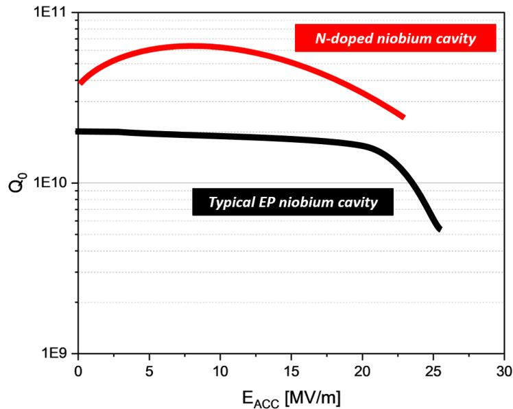
Figure 9.1: Comparison between typical electropolished niobium cavities and N-doped niobium cavities performances (figure after [31])
