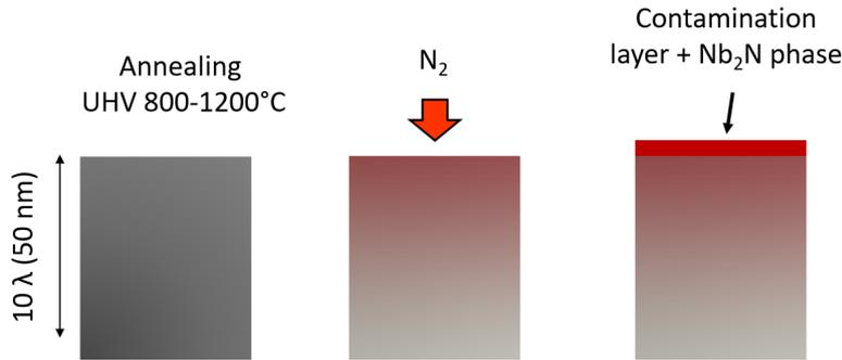
Figure 9.2: Illustration of the N-doping approach proposed by Fermilab
