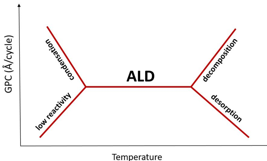
Figure 4.5: Atomic layer deposition temperature window
