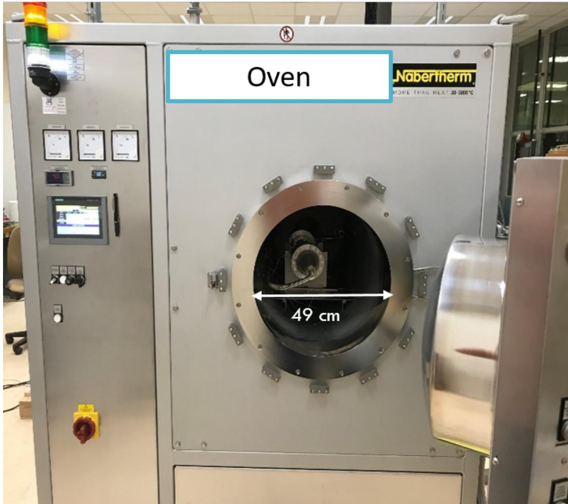
Figure 4.16: Picture of the retort of the oven
