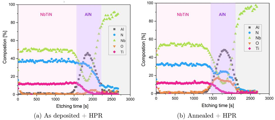
Figure 8.7: XPS profile of the Nb coated sample after the HPR treatment
