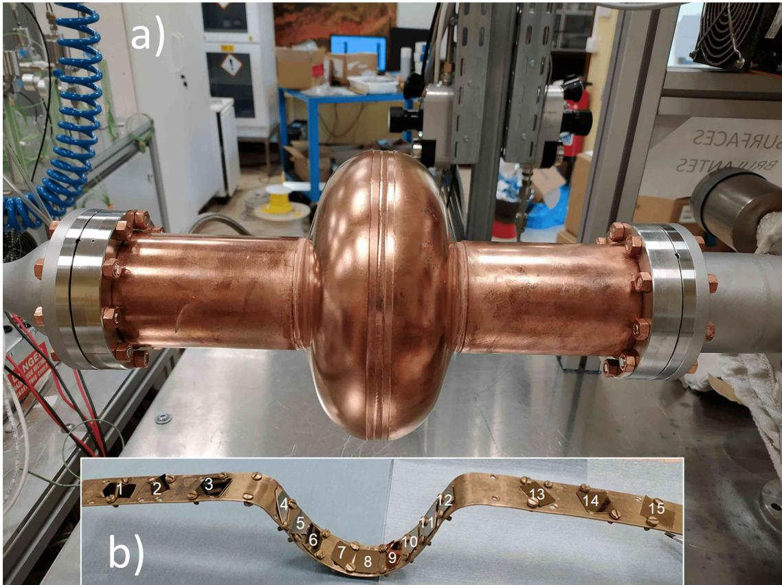
Figure 8.17: a) Picture of the copper cavity installed on the research-scale ALD system.
