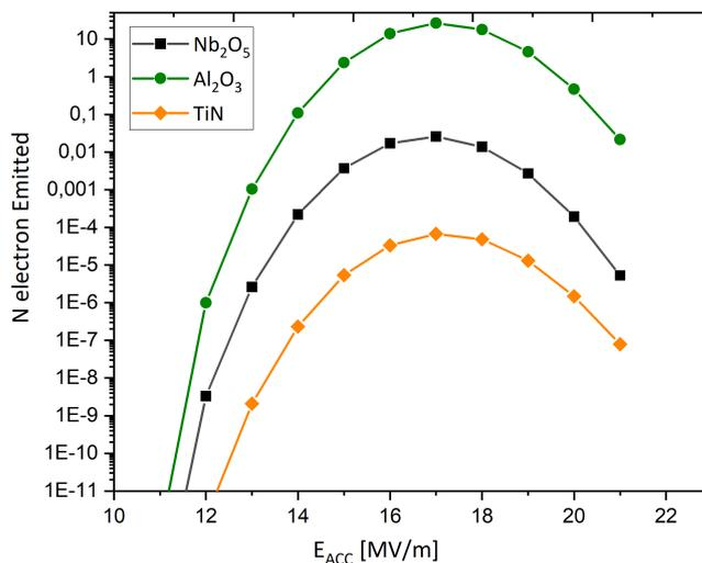
Figure 6.3: Calculated number of secondary electron emitted in a 1.3 GHz niobium cavity as a function of the accelerating field coated with Al<sub>2</sub>O<sub>3</sub>, TiN or with its native oxide Nb<sub>2</sub>O<sub>5</sub>
