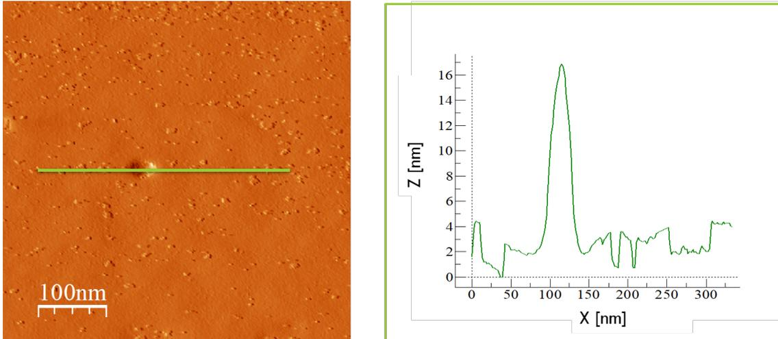
Figure 8.14: AFM scan on the bare niobium sample
