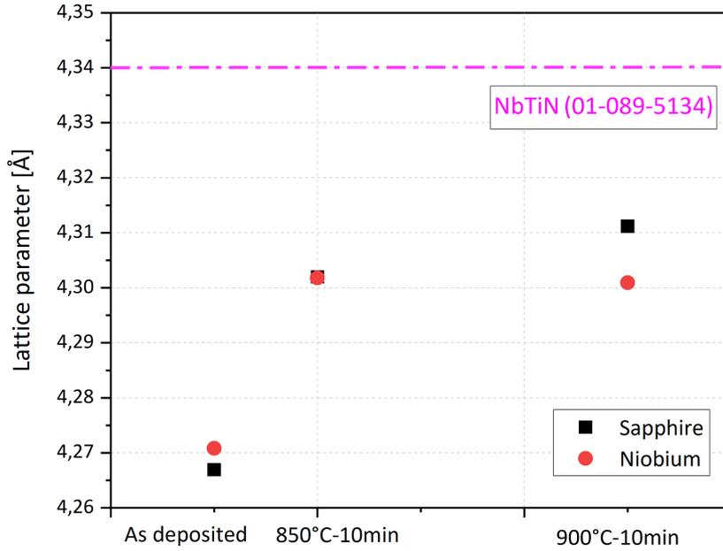
Figure 7.19: Evolution of the lattice parameter of the NbTiN film with 25% of Ti with different thermal treatment on Nb and sapphire substrates
