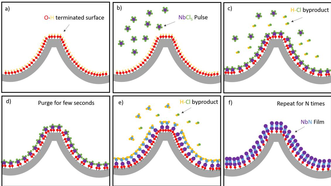
Figure 4.3: Schematic description of a niobium nitride ALD cycle
