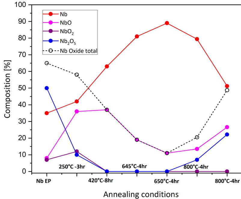
Figure 5.9: Summary of the Nb 3d core level composition of Al<sub>2</sub>O<sub>3</sub>-coated niobium
