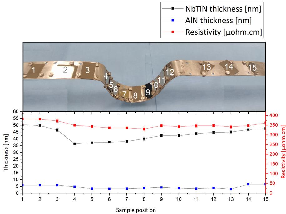
Figure 8.20: Results of the second test with 20 s purge for NbTiN film
