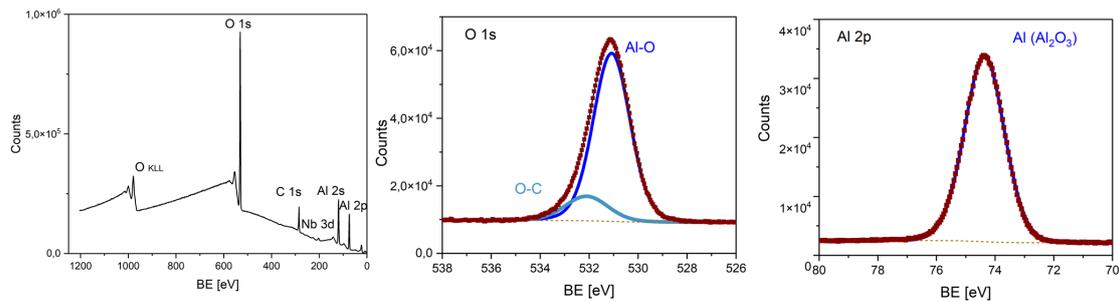
Figure 5.5: XPS analysis of 9 nm thick Al<sub>2</sub>O<sub>3</sub> film on niobium substrate
