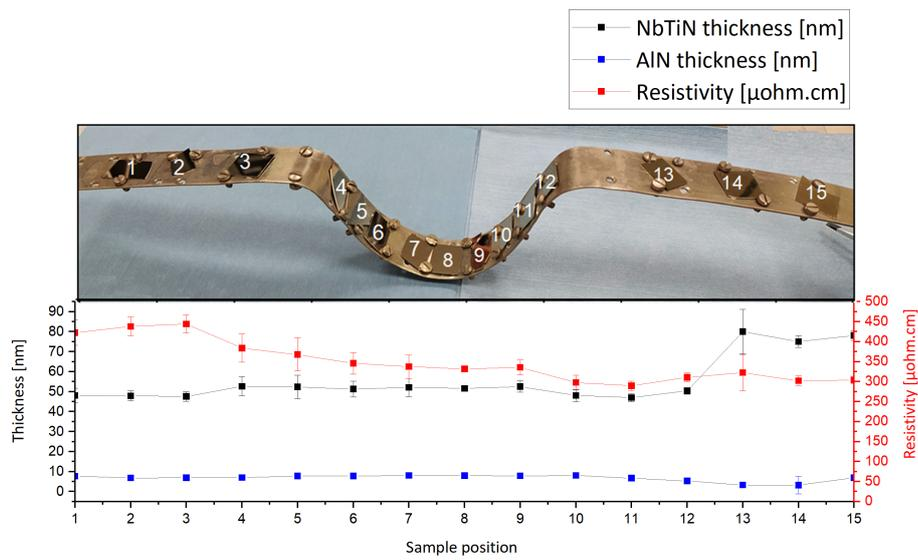
Figure 8.19: Results of the first test with 10 s purge for NbTiN film
