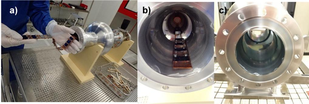
Figure 5.15: a) Pictures of the Aluminium cavity with the sample holder, (b) before the deposition, (c) the aluminum cavity after the deposition showing a blue shade characteristic of the  $\text{Al}_2\text{O}_3$  oxide layer
