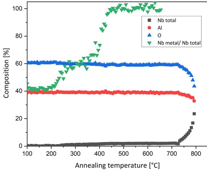
Figure 5.10: XPS analysis of Al<sub>2</sub>O<sub>3</sub>-coated Nb sample with in-situ annealing
