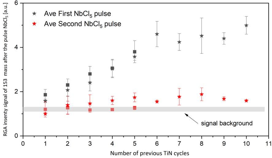
Figure 7.9: The intensity of the 153 mass as recorded by the RGA when we pulsed the NbCl<sub>5</sub> for the first time (in black) and for the second time (in red) as a function of the number of TiN cycles previously done
