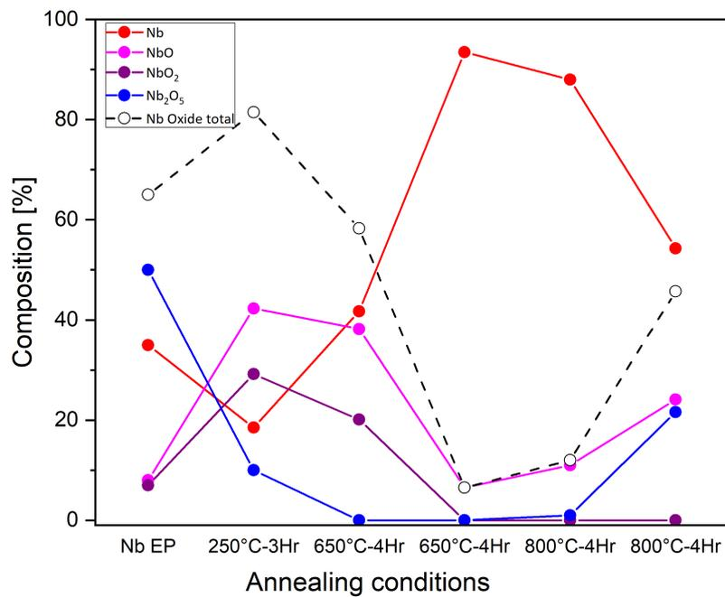
Figure 5.11: Summary of the Nb 3d core level composition of Y<sub>2</sub>O<sub>3</sub>-coated niobium
