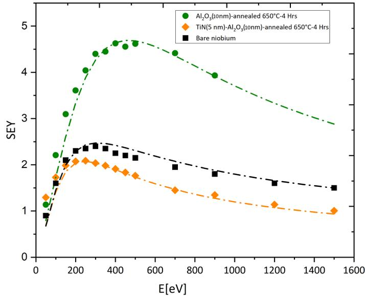
Figure 6.2: SEY measurement of a bare niobium surface,  $\text{Al}_2\text{O}_3$  coated niobium surface annealed during 4 hours at  $650^\circ\text{C}$  and TiN (5 nm) - $\text{Al}_2\text{O}_3$  (10 nm) coated niobium sample annealed during 4 hours at  $650^\circ\text{C}$ .
