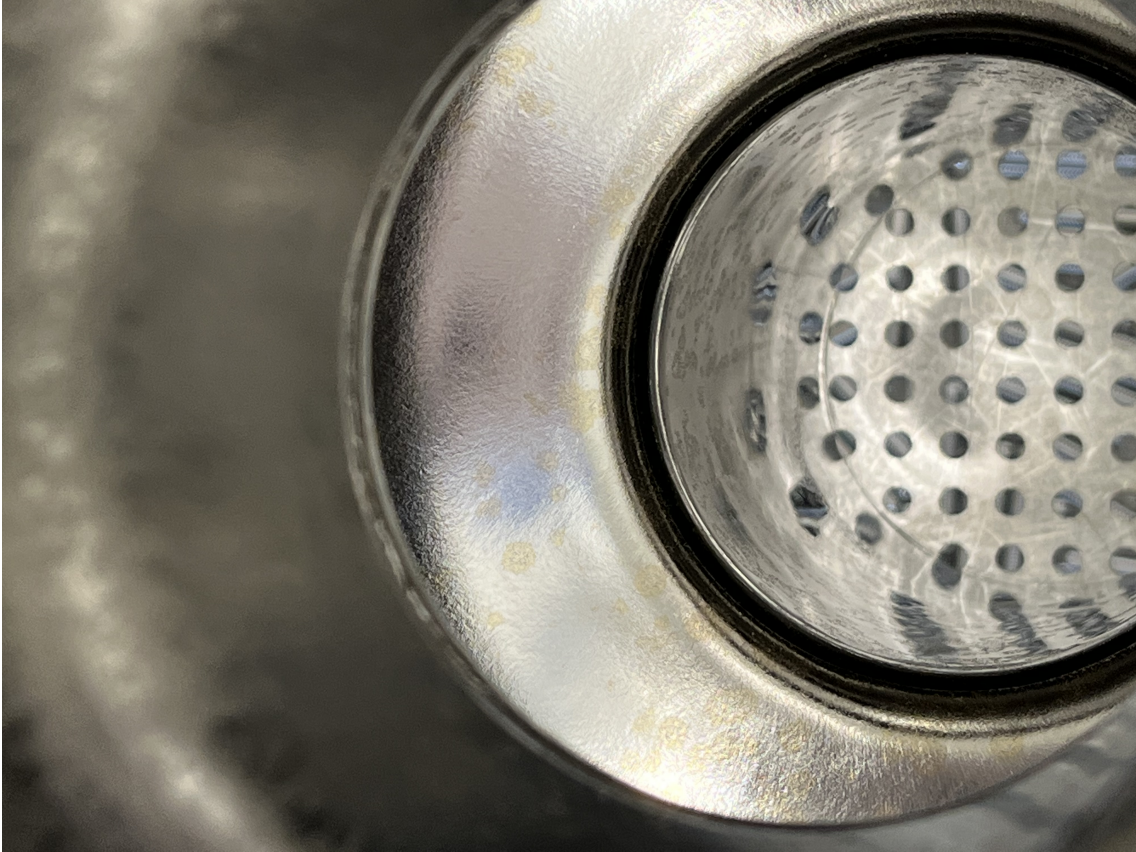
Figure 8.24: Picture of the cavity cell after the annealing
