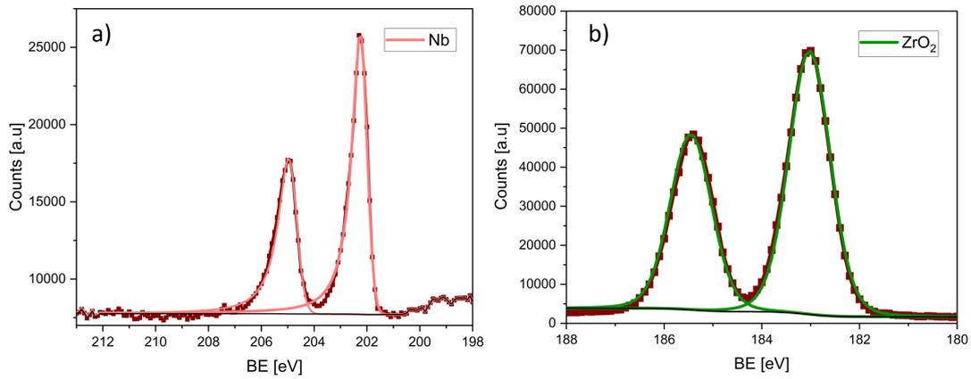
Figure 9.11: a) The Nb 3d core level spectra on the ZrN coated sample after annealing at 900°C-3 hours. b) The Zr 3d core level showing ZrO<sub>2</sub> contribution at BE =183 eV
