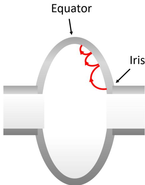
Figure 6.1: Multipacting trajectories in elliptically shaped RF cavities
