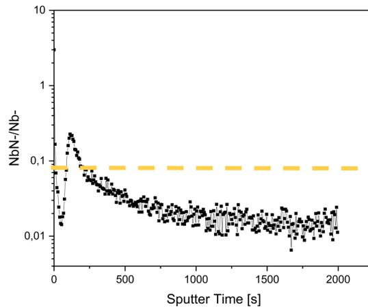
Figure 9.15: TOF-SIMS analysis on AlN coated Nb sample after ALD coating + annealing. The dashed line in yellow represents the NbN-/Nb- obtained with the conventional doping approach (after [130])
