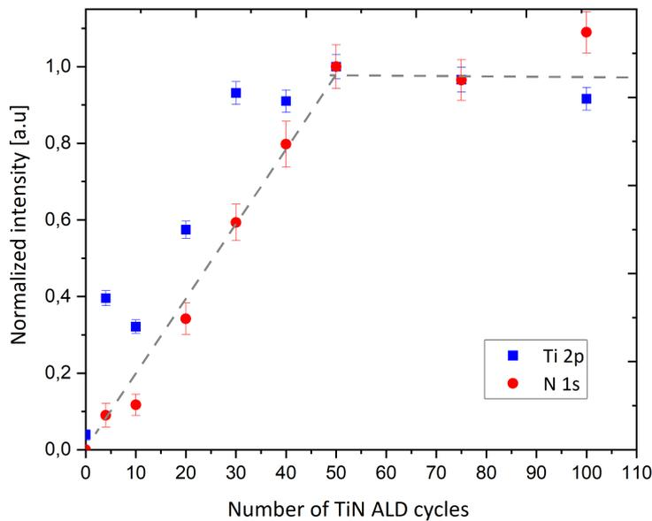
Figure 6.10: The XPS Ti-2p and N-1s intensities of the TiN-Al<sub>2</sub>O<sub>3</sub> coated Si samples with the number of TiN ALD cycles from 0 to 100
