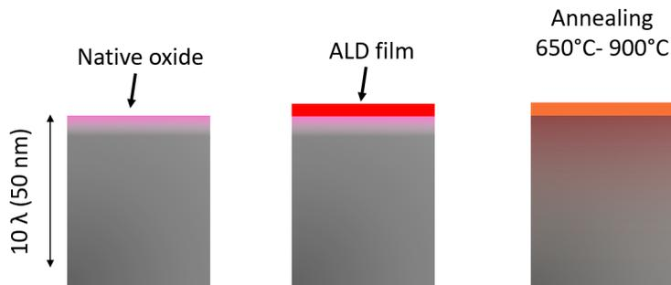
Figure 9.3: Illustration of the N-doping approach using ALD
