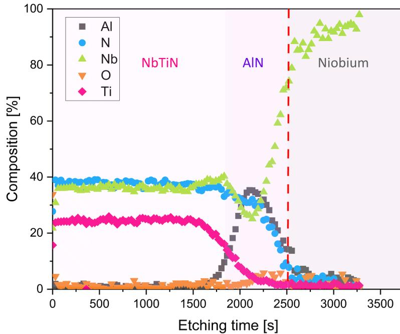
Figure 8.11: XPS profile of the NbTiN-AlN bilayer deposited on niobium using Ar as a transport gas for the ALD deposition
