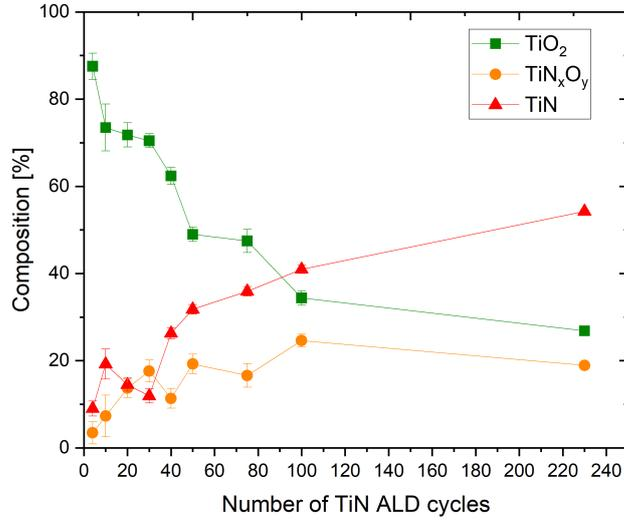
Figure 6.13: The chemical composition of the ALD-deposited TiN films as a function of the number of ALD cycles
