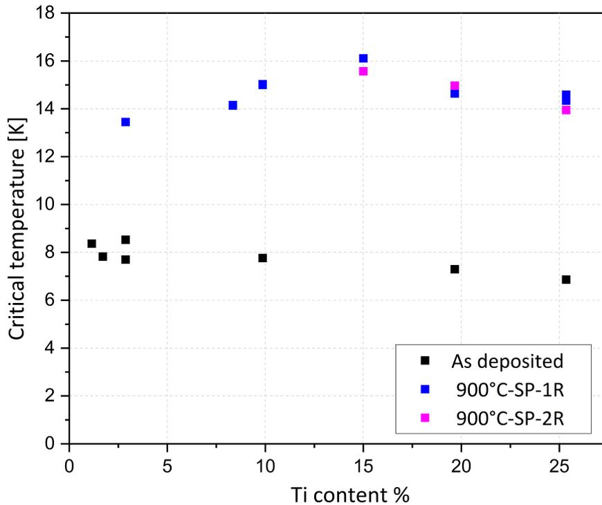
Figure 7.24: Critical temperature measured on 50 nm NbTiN films deposited on 10 nm AlN on sapphire substrates after annealing in vacuum
