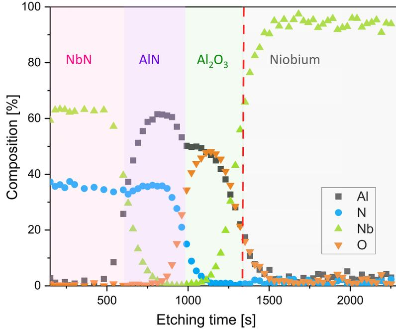
Figure 8.12: XPS profile of the NbN-AlN-Al<sub>2</sub>O<sub>3</sub> bilayer deposited on niobium using N<sub>2</sub> as a transport gas for the ALD deposition
