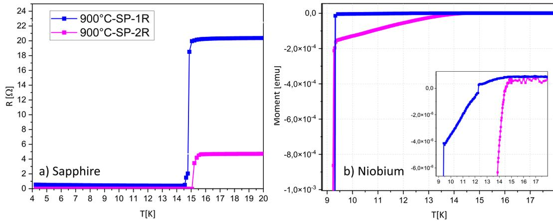
Figure 7.31: Critical temperature measurements on the NbTiN film (8:1)
