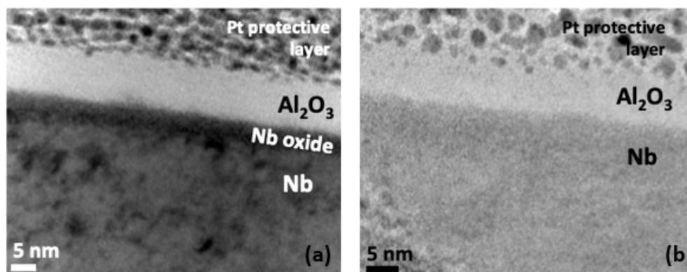
Figure 5.13: Transmission Electron Microscopy bright field images (JANNuS-SCALP facility at IJCLab) of  $\text{Al}_2\text{O}_3$  films deposited on niobium: (a) as-deposited, (b) after annealing at  $650^\circ\text{C}$  during 4 hours
