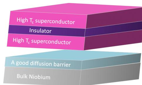
Figure 5.1: An illustration of the multilayer structure on top of the Nb surface protected by a diffusion barrier
