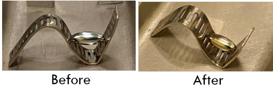
Figure 8.2: Picture of the niobium ellipsoid sample before and after the coating with AlN-NbTiN (6:1) films. The golden coloration is a typical sign of the presence of nitrides
