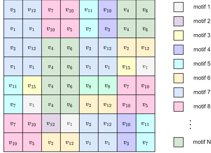
Figure 6.4 – Example of encoding an image into motifs. Initially, the quantized image is divided into tiles of 2 \times 2 elements. According to the block dictionary \mathcal{D}_b previously computed, the encoding into motifs will be performed by trying to encode the whole tiles first. Whenever it is not possible because the tile does not exist in the \mathcal{D}_b , the tile will be progressively divided into smaller blocks until all of them are assigned to a motif. In this example, each color correspond to a motif.
