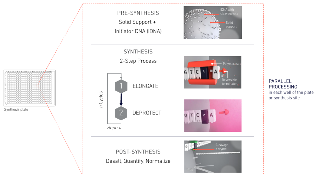
Figure 2.3 – Process of enzymatic DNA synthesis. Source: (DNA Script, 2022).
