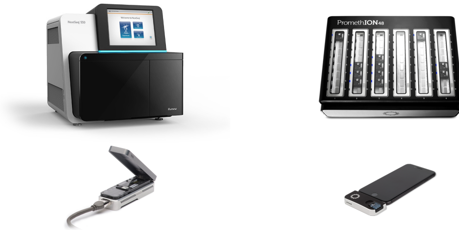
Figure 2.10 – Top left: Illumina NextSeq 550 (Illumina, s. d.). Top right: PromethION, bottom left: MinION and bottom right: SmidgION (ONT, s. d.).
