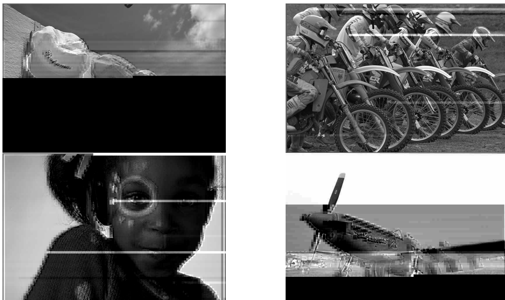
Figure 3.4 – Example of visual distortion on images encoded with the JPEG-inspired codec for DNA with 0.05% of substitution errors on the encoded DC coefficients.
