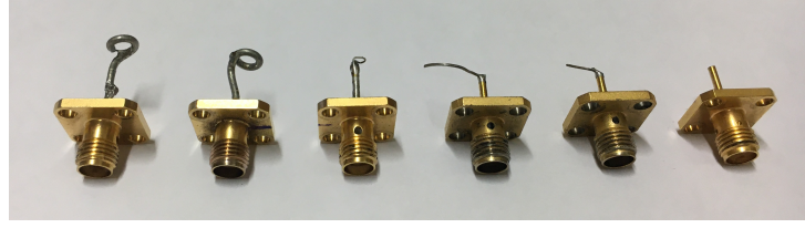
Figure 2.7 – Pictures of the different antennas that we use. From left to right: Two different loop antennas with big loops, a loop antenna with a small loop, a strongly coupled curved kink antenna, a weakly coupled straight kink antenna and a short monopole antenna.
