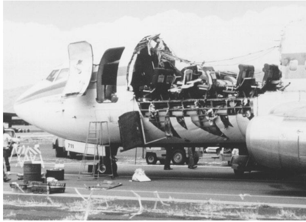
Figure I. 2. Fuselage failure in a passenger jet that occurred in 1988 (NASA TECHNOLOGY)
