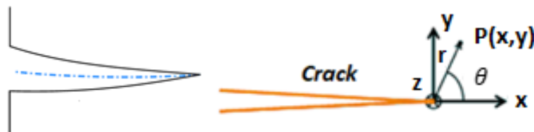
Figure I. 8. Separation of a medium on either side of an interface and the local reference frame attached to the fracture tip
