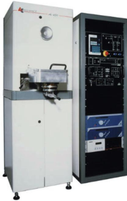
Figure II.4: Magnetron sputtering system available at INL: AC-450 by Alliance Concept.
