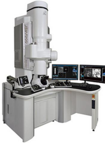
Figure II.13: TEM microscope JEOL JEM-200F used for HR-TEM experiments.
