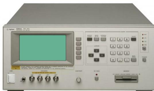
Figure II.23: HP 4284A Precision LCR meter.
