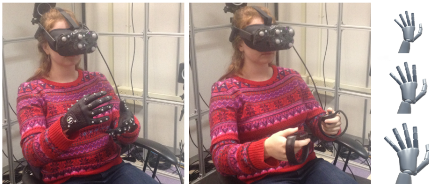
Figure 1.8 – Two different input modalities: hand tracking versus controllers. Hand tracking is preferred and better for the sense of embodiment. Image from [Lin et al. 2019].
