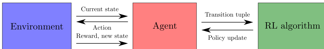
Figure 6.3: Generic Reinforcement Learning scheme. The agent interacts with its environment by "observing" the environment state s_t ; using its policy \pi , it acts on the environment through an action a_t = \pi(s_t) ; given this action, the environment updates its state, and the agent observes both the new environment state s_{t+1} and the reward r_t it obtained when performing its action. The resulting transition tuple \tau = (s_t, a_t, s_{t+1}, r_t) is then transmitted to the Reinforcement Learning algorithm, which updates the policy \pi accordingly in order to maximize the obtained rewards.
