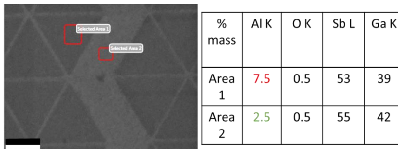
Figure.A.3. 9. EDX analysis of the SEM image of the physically etched HC transferred to the Al layer (area 1) and surrounded by the doped GaSb layer (area 2) grown on an undoped GaSb substrate. The scale bar is 10 \mu\text{m} long. As detailed in the associated table, Area 2 is revealing a considerable percentage of Al due to insufficient etching time.
