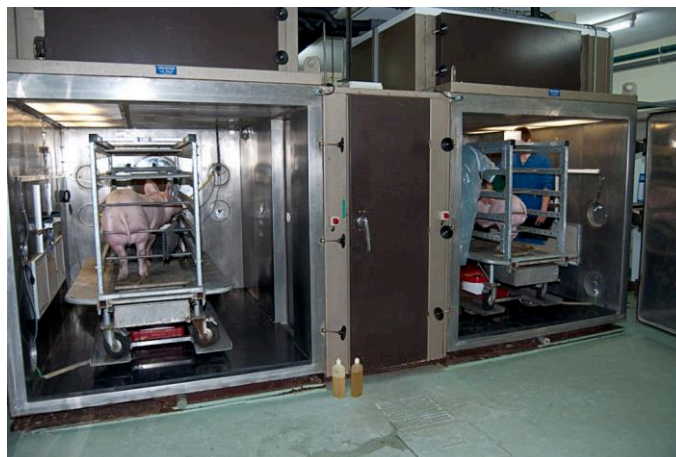
Photo 1: Two 12 m 3 open-circuit respiration chambers used in experiment 3 for nitrogen and energy balance measurements.
